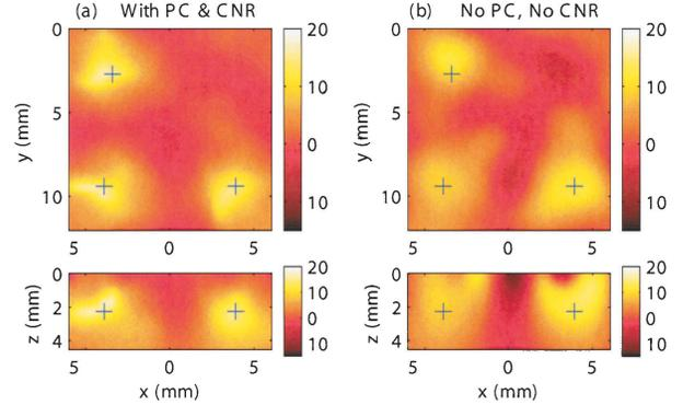
Fig. 2. Image reconstruction methods were evaluated with simulations. (a) CNR in  $\delta\mu_a$  with PC and SV-CNR weighting,  $xy$  slice at  $z = 2.25$  mm and  $xz$  slice at  $y = 9.5$  mm. (b) CNR in  $\delta\mu_a$  without PC and without SV-CNR (e.g., constant) weighting. Color bars state CNR.
