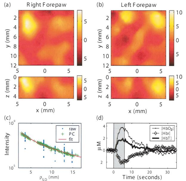
Fig. 3. Experimental DOT images of CNR in  $\delta\mu_{a,\lambda=830\text{ nm}}$  during rat brain activation. (a) Right forepaw,  $xy$  slice at  $z = 1.75$  mm,  $xz$  slice at  $y = 2$  mm. (b) Left forepaw,  $xy$  slice at  $z = 2.25$  mm,  $xz$  slice at  $y = 2$  mm. (c) Calibration of optode positions by use of baseline intensities. (d) Activation time traces of [HbR], [HbO<sub>2</sub>], and [HbT].
