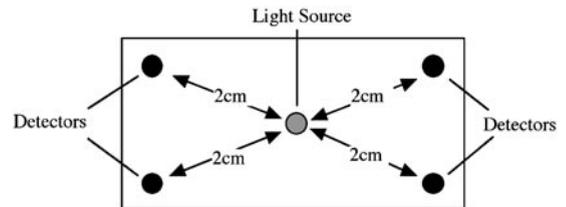
**FIG. 1.** Schematic diagram of the NIRS probe. A single 1-mm bifurcated light source is located centrally, surrounded in a rectangular formation by four 1-mm detectors.
