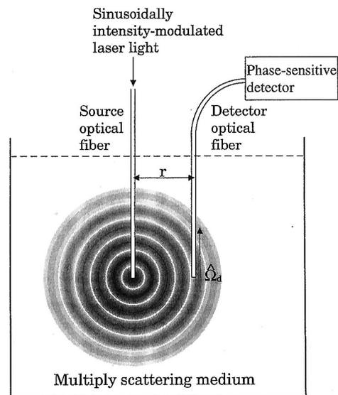
Fig. 2. Typical geometry used to generate and detect a diffusive photon-density wave.  $\hat{\Omega}_d$  is the principal direction in which photons can enter the detector optical fiber. We assume that a Dirac-delta function  $\delta(r)$  accurately describes the light source when  $r \gg 1/\mu_s'$ .
