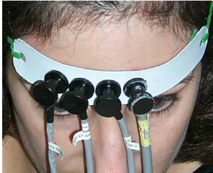
Figure 4.12. A photo of the optode assembly used to perform the Valsalva measurements. Separate 3mm diameter silica fiberoptic bundles were used to couple light from three 830nm laser diode sources to the forehead, and back to the silicon detector (thick bundle on far right). The fourth source was not used for these measurements. The assembly was placed on the forehead as shown above and held in place with an elastic band. All four optodes were spaced by approximately 16mm, and the radius of curvature was about 80mm.
