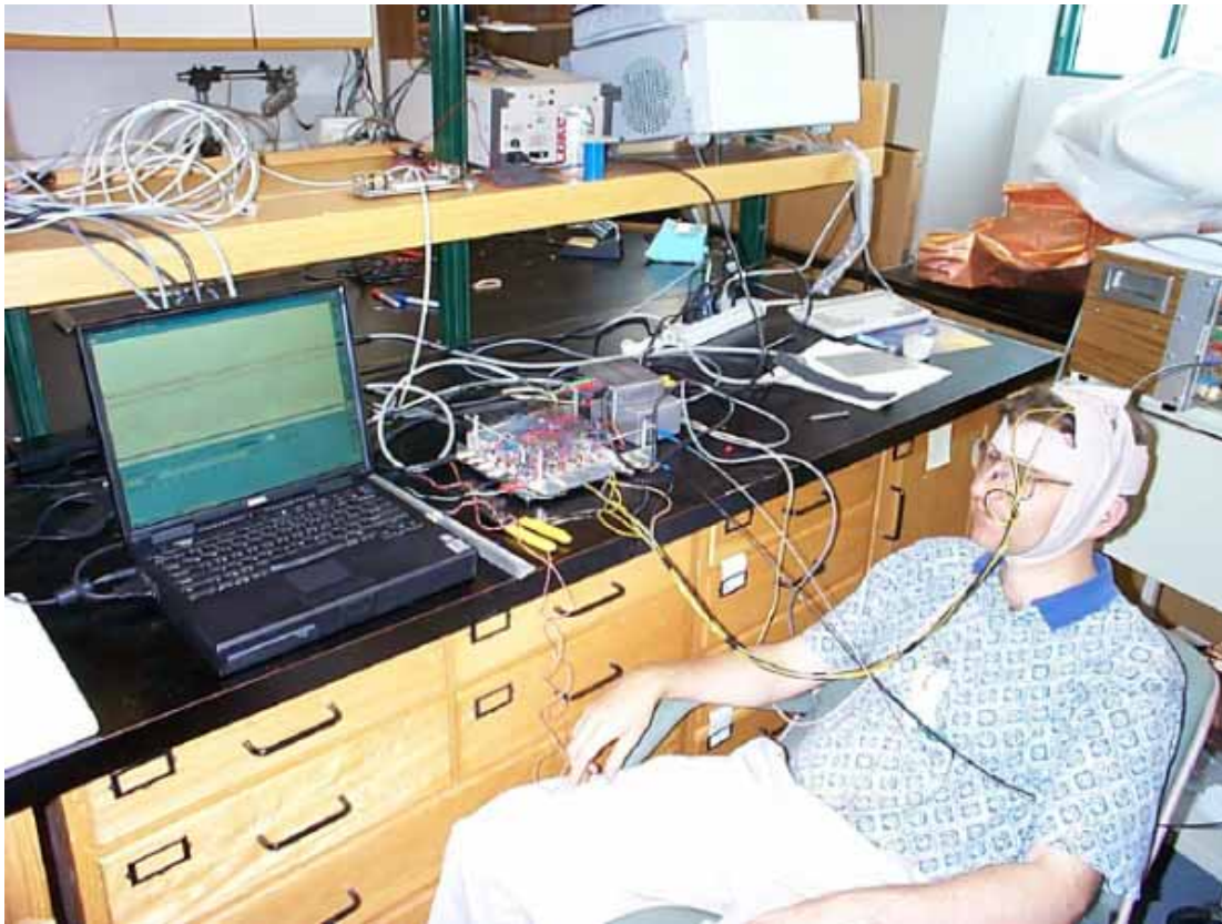
Figure 4.23. An image showing Gertrude in use. The gray die-cast boxes enclosed the high-power 808nm laser source and an electrolytic strain gauge respirometer which was used to monitor ventilation. The three OPT209 detectors were located on the optode assembly and were optically coupled to the scalp through light pipes constructed from 1cm lengths of 3mm diameter PMMA fiber.
