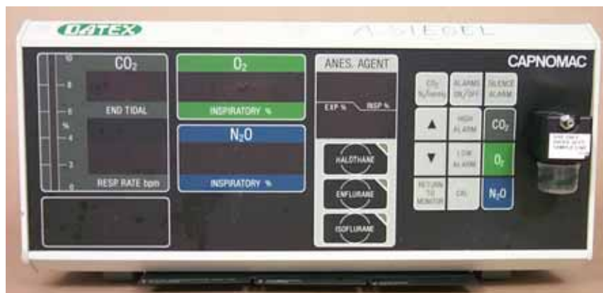
Figure 5.15. This Datex Capnomac anesthesia monitor, obtained at nominal cost from the MIT Flea Market with some mechanical damage, was repaired and used primarily for capnometry measurement.
