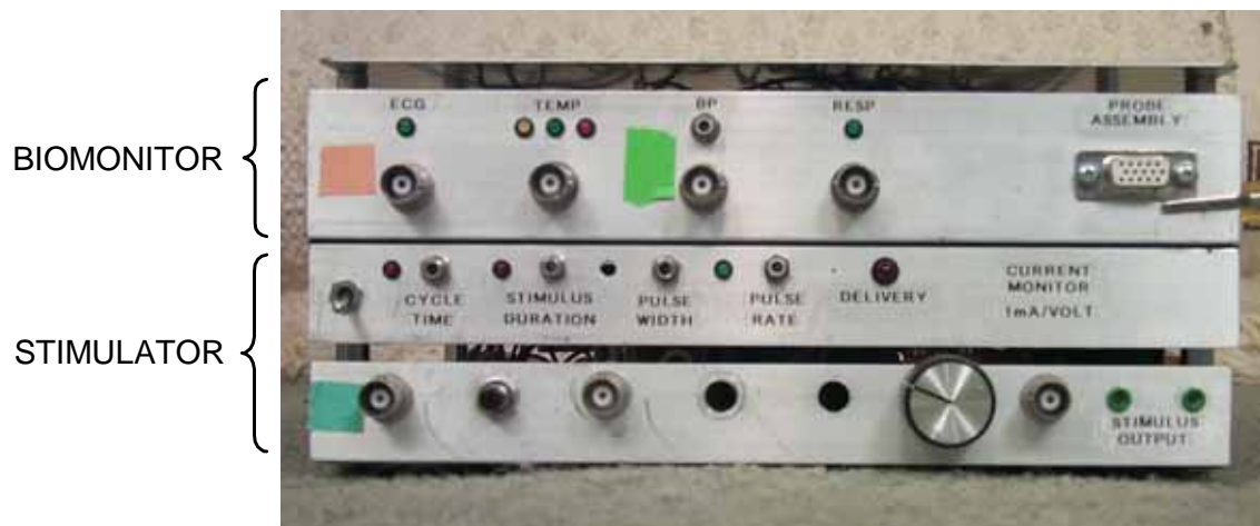
Figure 5.10. A front panel view of the biomonitor unit, which is shown mounted above the forepaw stimulator. Both circuits share a common +/- 12V power supply module and utilize a common chassis ground. Colored tape indicates specific BNC cable connections to the analog data acquisition system.
