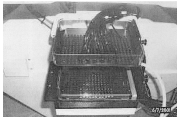
Fig. 6. Compression plates with fibers of our clinical breast imaging system. The plastic plates are standard mammography plates modified to hold our optical fiber arrays. The sources are on the bottom plate and fill roughly the middle third of the plate (only the ends of the fibers are clearly visible). Detector fibers can be seen coming out of the top plate. The imager electronics are to the right, outside the photo.
