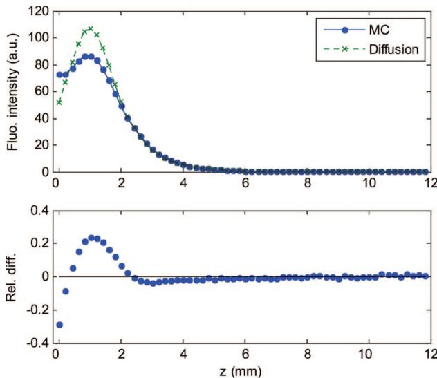
Fig. 3. (Color online) Fluorescence intensity calculated by the MC and the DA (upper panel) and the relative difference of the MC and the DA (lower panel) for a point fluorophore positioned horizontally midway between the source-detector pair at various depths inside the medium. The source-detector separation is 3 mm.
