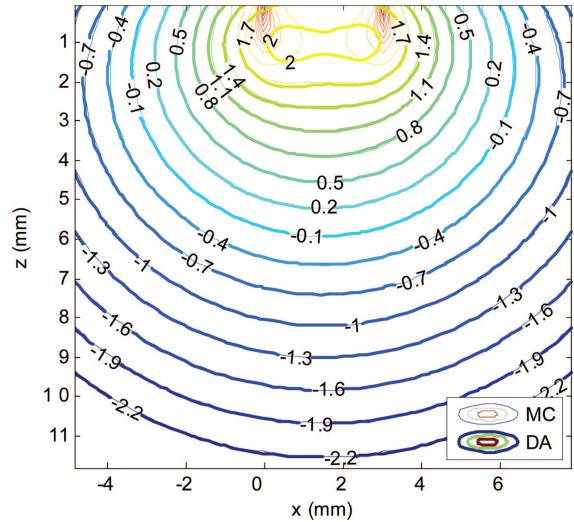
Fig. 2. (Color online) Comparison of the fluorescent intensity reaches the detector at  $(3, 0, 0)$  for a point fluorophore placed in a single pixel at various positions  $(x, z)$  in the  $x$ - $z$  plane excited by a unitary impulse light source injected at  $(0, 0, 0)$  calculated by the simplified MC and the DA for the configuration geometry shown in Fig. 1.
