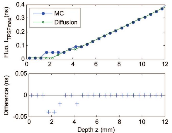
Fig. 5. (Color online) Time position of a fluorescence TPSF peak calculated by the MC and the DA (upper panel) and the difference of the MC and the DA (lower panel) for a point fluorophore positioned horizontally midway between the source-detector pair at various depths inside the medium. The source-detector separation is 3 mm.
