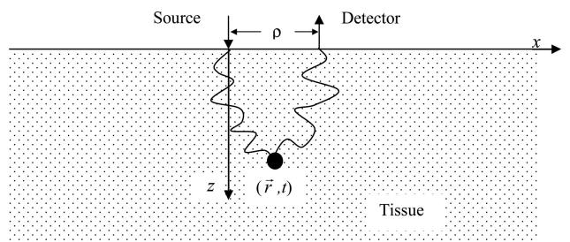
Fig. 1. Schematic of fluorescence spectroscopy in turbid medium such as biological tissue when reflection geometry is used.
