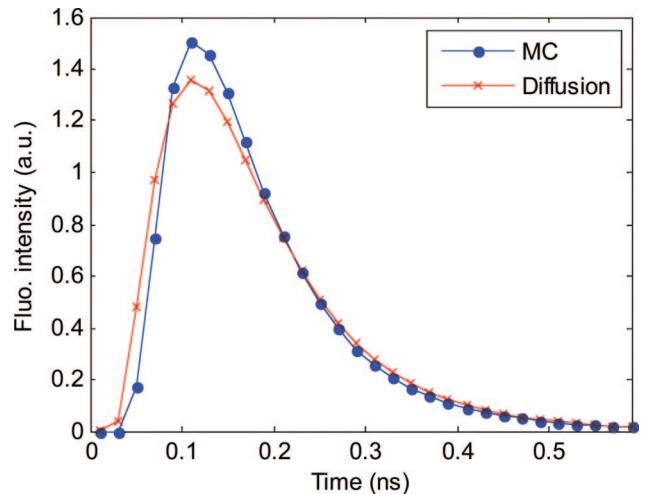
Fig. 4. (Color online) TPSF from a fluorescence signal calculated by the MC and the DA for a point fluorophore positioned horizontally midway between the source-detector pair at depth  $z = 5.25$  mm inside the medium. The source-detector separation is 3 mm.
