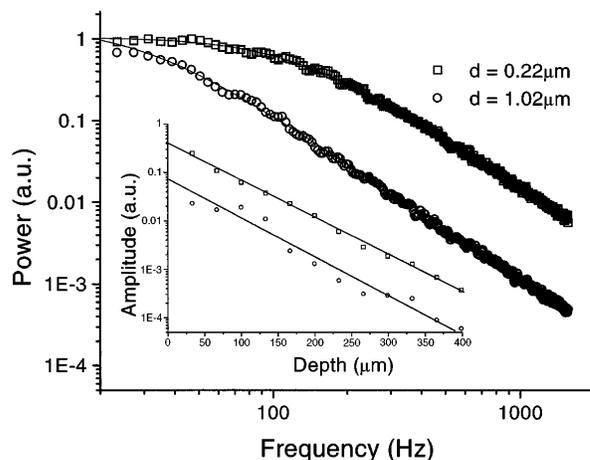
Fig. 2. Power spectra measured at a depth of  $200 \mu\text{m}$  for two different suspensions. The solid curves show the Lorentzian fits to the experimental data. Inset, amplitude as a function of depth in the sample for the same samples; the solid curves represent the expected amplitude decays.
