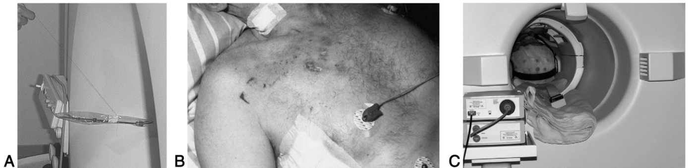
Fig. 3. (A) Magnetically-induced force attracting a metallic probe towards the magnet. According to standard safety criteria the deflection angle needs to be less than 45°. Reproduced from Schaeffers (2008) by permission of the copyright holder, IEEE. (B) Second-to-third degree burns on the thorax where ECG electrodes were applied, following an incident involving high-voltage induction in long leads. Reproduced from Kugel et al. (2003) by permission of the copyright holder, Springer-Verlag. (C) Reducing lead length, running the conductive wires in parallel near the centre of the magnet and using appropriate padding minimizes risks and improves signal quality. Reproduced from Herrmann and Debener (2008) by permission of the copyright holder, Elsevier.
