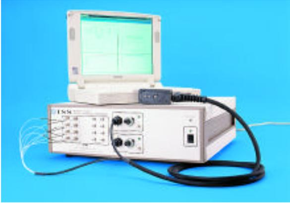
**Figure 2** Photograph of the frequency-domain tissue oximeter. Two synchronized tissue oximeter units were used (which provide a total of four parallel detection channels and 32 multiplexed light sources) for functional near-infrared imaging (fNIRI) of the brain (photograph courtesy of ISS, Inc.).
