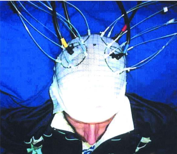
**Figure 3** Optical helmet used to arrange the 32 illuminating optical fibers and four collecting optical fibers on the head of the subject. The helmet and fiber optic cables contain no metal; thus this setup is suitable for concurrent optical and fMRI brain imaging.
