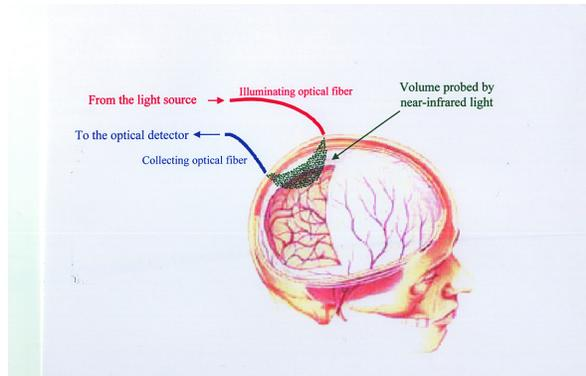
**Figure 1** Schematic representation of the noninvasive approach to the optical study of the brain. The light delivered to the skin by an optical fiber penetrates through the scalp and skull and probes the cerebral cortex before reaching the collecting optical fiber. The distance between the illuminating and collecting fibers is typically 3–4 cm. Near-infrared imaging of the brain involves the use of multiple pairs of source and detector optical fibers.
