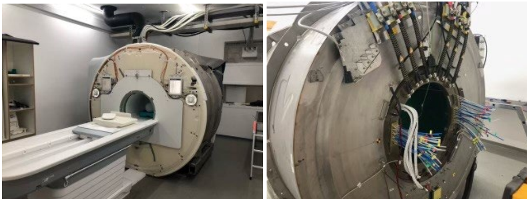
Figure 1. Photographs of the next-generation Siemens 3T Vida MRI system equipped with a high-performance whole-body gradient coil ( G_{\max}=200 mT/m, slew rate 200 T/m/s). Front (left) and back views (right) of the scanner show the gradient set integrated into the bore of the magnet and driven by two gradient power amplifiers.
