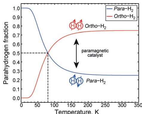
**Figure 8.** Parahydrogen conversion. Passage of H<sub>2</sub> gas over a paramagnetic catalyst, given sufficient contact time, converts the *ortho*-H<sub>2</sub> fraction to *para*-H<sub>2</sub> fraction as a function of temperature.
