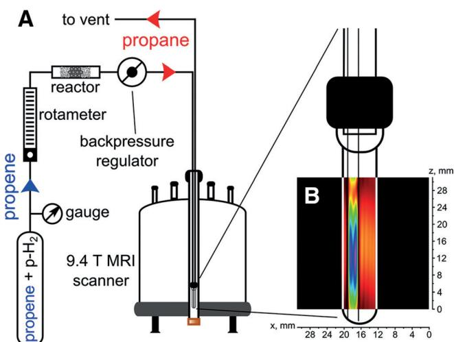
**Figure 12.** (a) Schematic representation of the experimental setup for using PHIP to produce HP propane via heterogeneous hydrogenation of propene with parahydrogen. (b)  $^1\text{H}$  MRI FLASH image of HP propane flowing into a 10 mm NMR tube via 1/16 in. OD Teflon capillary. Note that the NMR tube is shown schematically and its length does not match the actual scale of the 2D MR image. Reprinted with permission from ref. [220].
