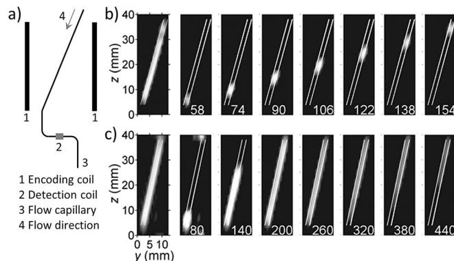
**Figure 15.** a) RD MRI setup of a simplified microfluidic system consisting of a capillary leading through the encoding and detection coils. TOF RD MRI visualization of (a) HP propane and b) water flow in the capillary (outlined in white), revealing much more extensive dispersion of liquid than that of gas molecules. TOF (ms) is shown at the bottom of the panels. The panels on the left are sums of the other panels.<sup>[230a]</sup>
