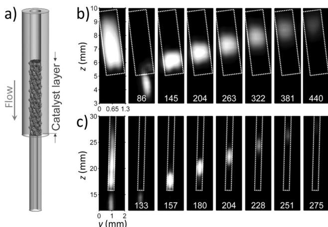
**Figure 17.** RD MRI visualization of reaction progress inside a catalyst layer packed in a thin capillary. a) Sample setup. 2D TOF images of HP propane resulting from the hydrogenation reaction in the reactors of a) 800 and b) 150  $\mu\text{m}$  in diameter. The reactors are outlined by a white dashed line in the figures. TOF (ms) is shown at the bottom of the panels. The panels on the left are the sums of all other panels in each series.<sup>[230c]</sup>
