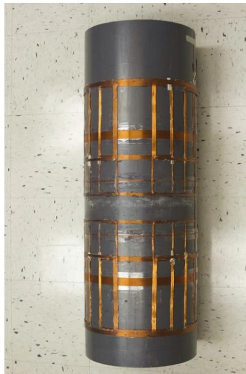
**FIGURE 5** Gradient coils for the low-field magnetic resonance imaging (LF-MRI) magnet. Z gradient coils were wound directly onto the plastic polyvinyl chloride (PVC) pipe, while X and Y gradient coils were constructed using a form and attached later. The gradient coils are located between the magnet and the radio frequency coil
