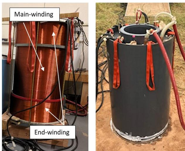
**FIGURE 4** The magnet (left) was constructed on a stainless-steel bobbin, wound with copper wire. The gray plastic polyvinyl chloride (PVC) housing (right) used recirculating oil to cool the magnet
