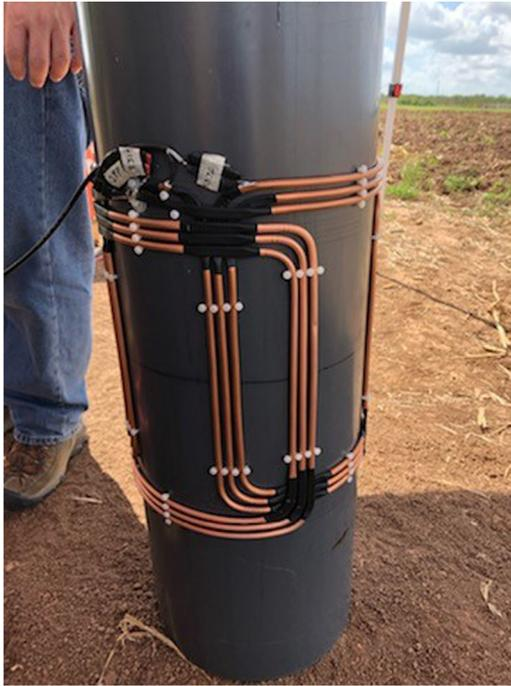
**FIGURE 6** The radio frequency coil was constructed using a quadrature design with X and Y direction saddle coils and was wound on 28.9 cm plastic polyvinyl chloride (PVC) pipe
