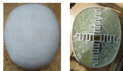
Fig. 14. Head-shaped structured phantom and internal structure.
