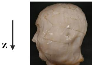
Fig. 5. Head-shaped liquid filled phantom. This phantom was filled with an aqueous solution of 9% NaCl and 1% Gd in DI.
