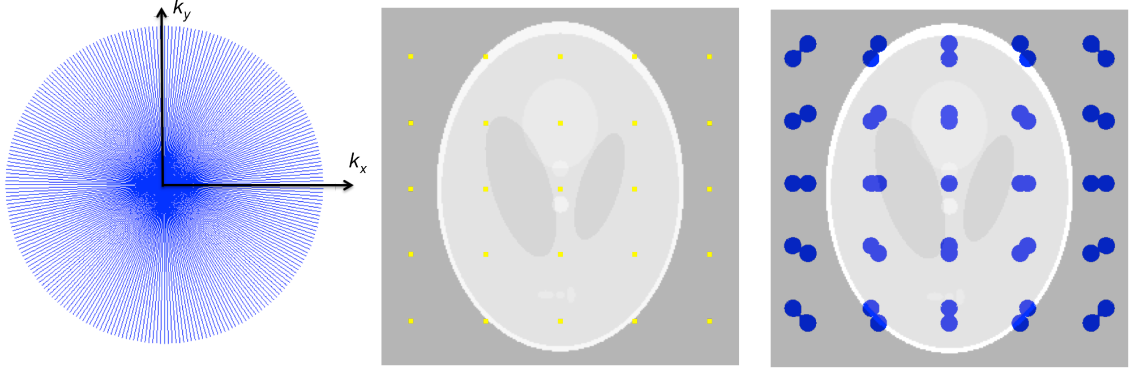
Figure 2.7: Local k-space trajectories for a representative 5 \times 5 grid of voxels from different sections of the FOV. The trajectories correspond to the O-Space readouts for the center placements shown in Fig. 2.5. At left is a conventional radial k-space trajectory corresponding to the center of the FOV, where the Z^2 SEM has zero amplitude, imparting no \mathbf{k}_{shift} . Elsewhere in the FOV, the Z^2 applies a \mathbf{k}_{shift} vector, altering the shape of k-space (and the resulting resolution) on a voxel-wise basis. The k-space plots do not include the effects of RF coil encoding.
