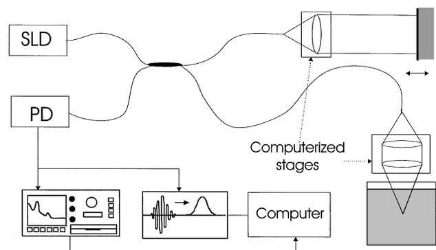
Fig. 1. Dynamic low-coherence interferometer system: PD, photodetector; SLD, superluminescent diode.
