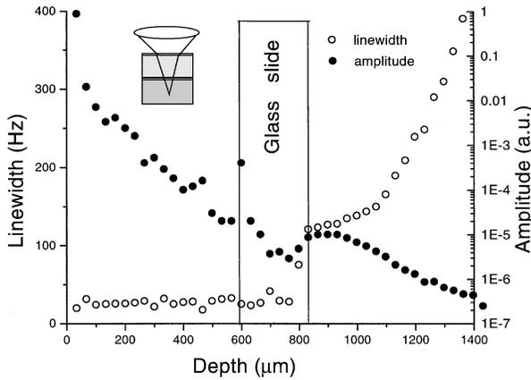
Fig. 4. Lorentzian linewidth and amplitude as functions of depth in the two-layer system. Inset, schematic of the cell used to image spatial variations in the dynamic properties of turbid media. Top layer, 0.5% suspension of 1.02- $\mu\text{m}$  PS spheres; bottom layer, 4% suspension of 0.22- $\mu\text{m}$  PS spheres.
