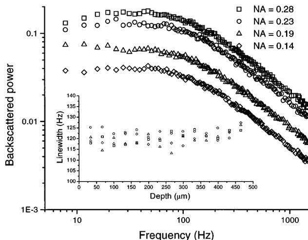
Fig. 3. Power spectra for a 4% monodisperse solution of  $0.22\text{-}\mu\text{m}$ -diameter PS microspheres for different N.A.'s of focusing objective. Inset, Lorentzian linewidth as a function of depth for different N.A.'s of the focusing objective.
